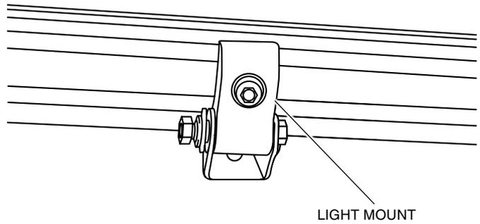
3. Install the appropriate size light clamp to the light mount.
