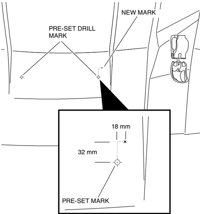
5. Drill a 3/4 inch hole at the new mark with a step drill.
