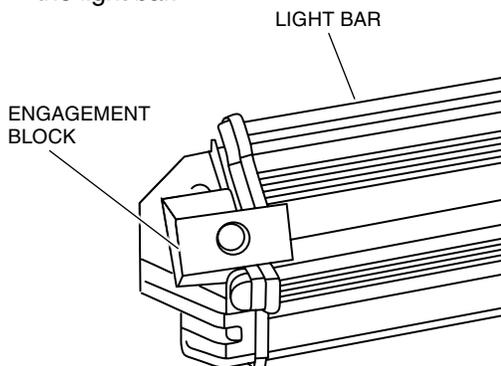
2. Attach the light mount to the engagement block with the included bolt.
