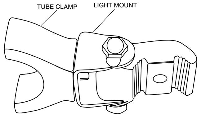
4. Install the assembled light bar/clamp assembly to the desired location on the cab frame or bumper tube.
