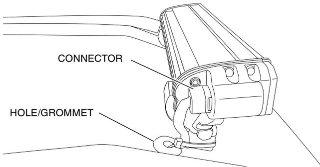
2. Route the wire lead along the upper cab frame cross tube and then down the right front A-pillar.
