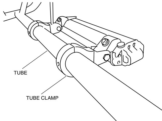
5. Adjust the light bar to the desired beam angle.
