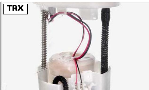
26. Install the fuel sender into the reservoir.
