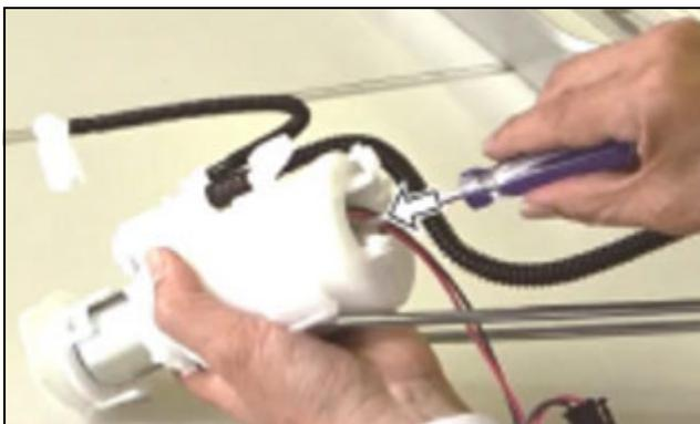
17. Remove the wire harness and spacer from the fuel pump.
