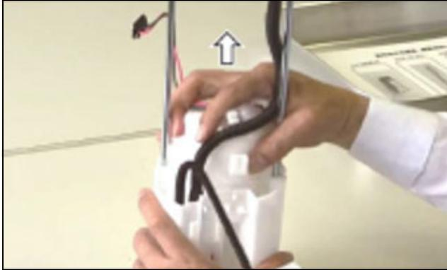
15. Remove the fuel pump by releasing the three lock tabs in the locations shown.
