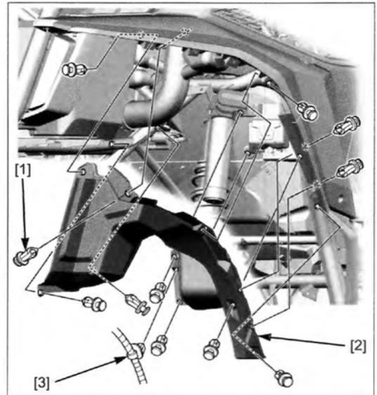
2. Remove the OEM air intake snorkel (1) from the air box inlet and remove the flexible inner fender seal curtain (2) attached to the fender and OEM snorkel. \*
